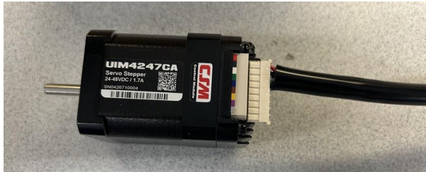
Figure 4-1. The keyed motor connector seated on the motor (wire colors aligned to the connector legends).
