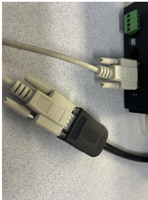
Figure 4-2. The supplied 3-ft DB9 cable connects the motor cable to the MOTOR port; secure the thumbscrews at both ends.
