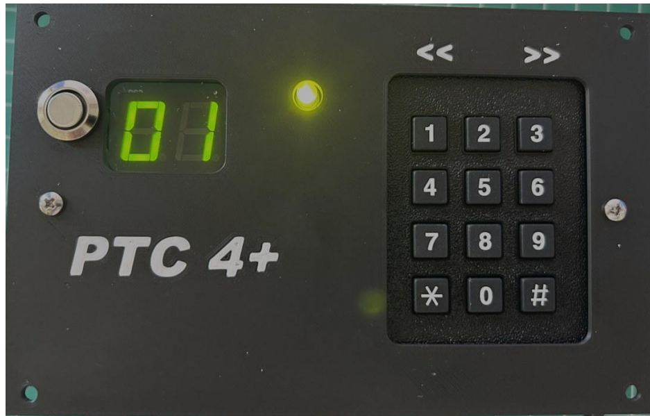
The PTC Model 4+ front panel: power button, TRACK display, status LED, and keypad. (Shown: 3D-printed beta panel; production panels are black anodized aluminum.)
