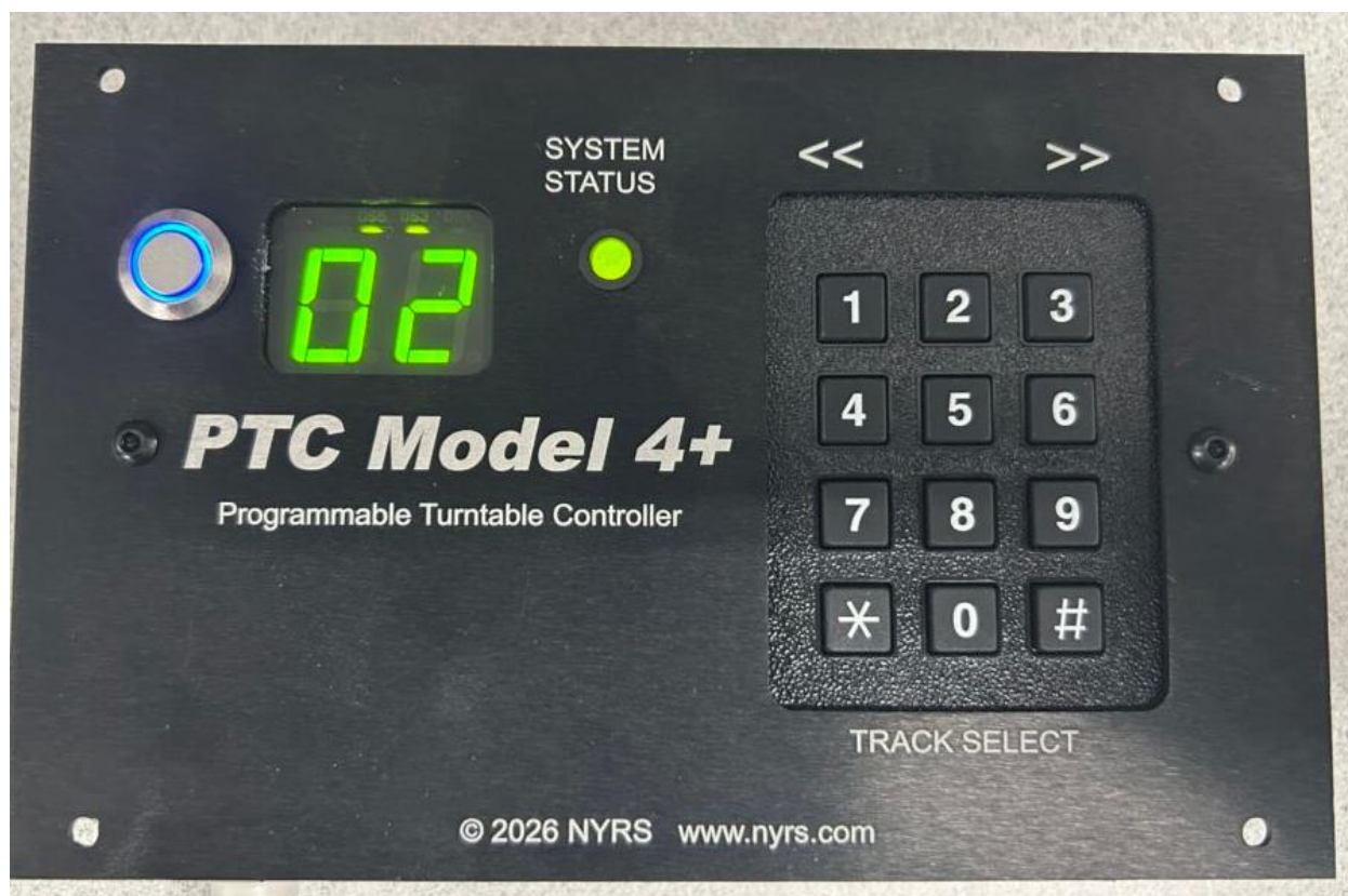
The PTC Model 4+ front panel: power button, TRACK display, status LED, and keypad
