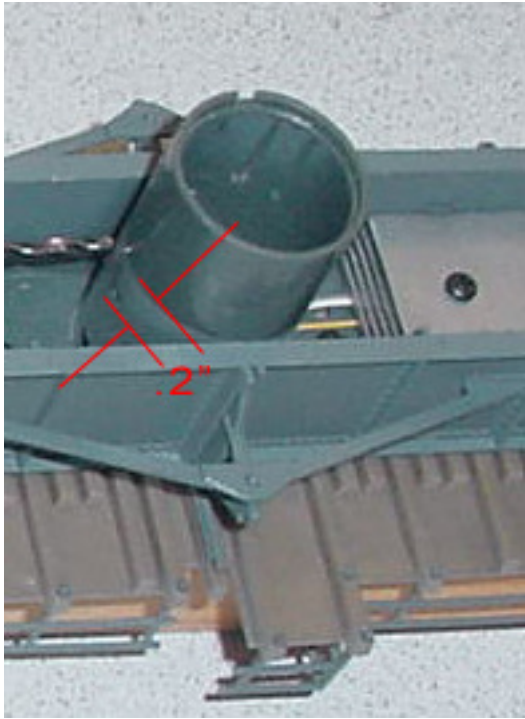
Figure 6a: Hole placement
